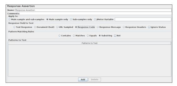
For our purposes, we will use the **Response Assertion** component. The panel enables us to compare various fields of the response. Using this, we can verify the response text, response code, response headers, and so on.
