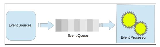
When compared with the thread-based architecture, EBA gives better performance output. In EBA, there are a fixed number of threads performing tasks and no new threads are formed. Thus, we achieve better utilization of the CPU and an improved memory footprint. There is also no overhead of excessive context switching and no need for a thread stack for each connection. Ideally, the CPU becomes the only apparent bottleneck of an event-driven application.
