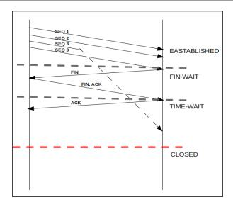
The long TIME\_WAIT state results in the memory and ports getting blocked by closed connections. Thus, a heavily loaded server can run out of resources, which can be caused by a large number of connections in the TIME\_WAIT state.
