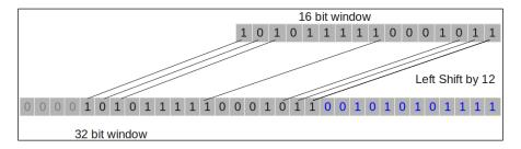
The buffer allocated at the receiving end is dynamically altered by the value in this window field. Window scaling is part of the TCP handshake and is enabled by default. This feature of TCP can be toggled using net.ipv4.tcp\_window\_scaling.
