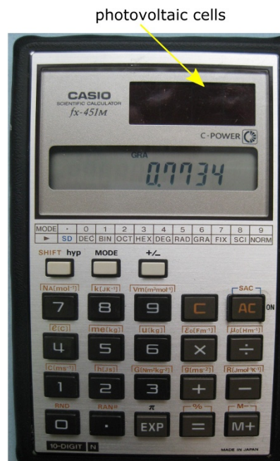
Figure 1-8: This calculator is powered by photovoltaic cells.
