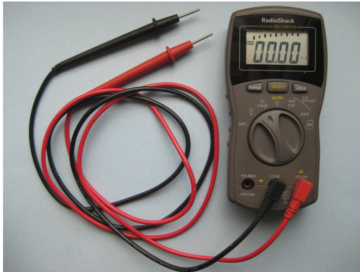
Figure 16-1: Multimeters measure voltage, resistance, current, and continuity.
