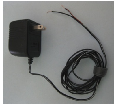
Figure 12-6: This AC adapter converts 120 volts AC to 7.5 volts DC and supplies up to 300 mA of current. I modified the output of this adapter to make it easier to use in DC circuits.
