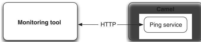
Figure 12.1 A monitoring tool monitors Camel with a ping service by sending periodic HTTP GET requests.
