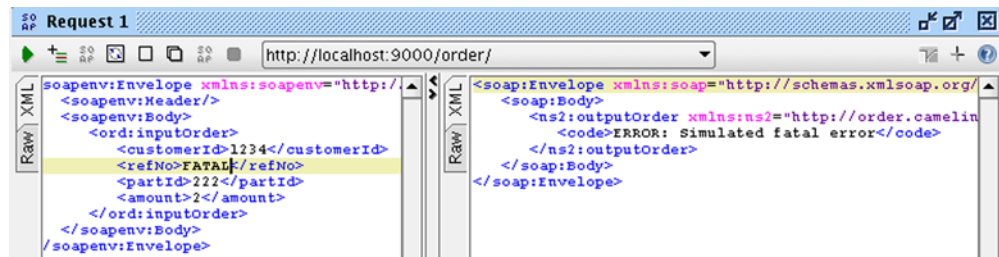
Figure 9.12 A web service message causes the transaction to roll back, and a custom reply message is returned.
