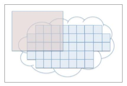
Note that this strategy approximates arbitrary shapes by using a grid of smaller shapes at an index time. This method basically allows the strategy to support any shapes. A match is when a searching query shape intersects with any shapes in the index. The preceding diagram is reflective of RecursivePrefixTreeStrategy. TermQueryPrefixTreeStrategy is slightly different; it indexes points instead of shapes for closer approximation at the expense of larger index and slower query.
