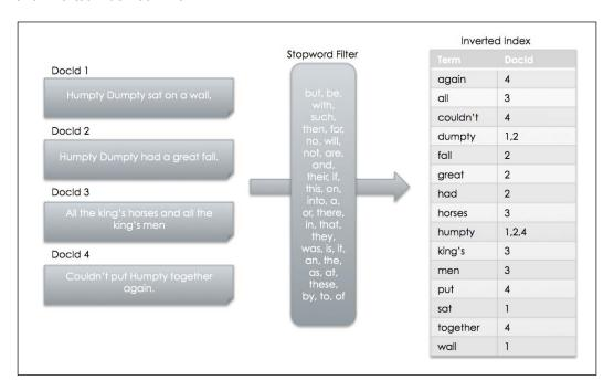
The preceding diagram illustrates that the Analyzer filters out stopwords and the resulting tokens, generated by the tokenization process, are extracted and stored as individual terms. Note that the inverted index contains a sorted list of terms with an associated Docld for each term. The term to Docld relationship is a one-to-many relationship. The analysis process and the inverted index are important concepts for understanding how to use Lucene effectively.
