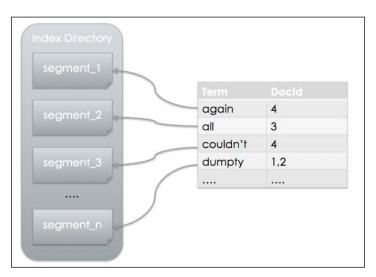
The terms and documents can exist in any of the segments, depending on when the new documents and terms are added. The IndexReader attributes will merge the index segments internally so that you can access a coherent index without having to consider the index segmentation.
