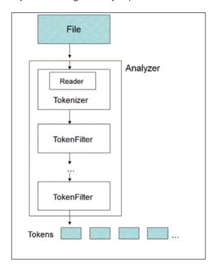
In this illustration, a tokenizer uses a reader object to consume text. It produces a sequential set of tokens that is called **TokenStream**. **TokenFilter** accepts the TokenStream, applies the filtering process, and emits filtered data in TokenStream in return. TokenFilters can be chained together to attain the desired results. A character filter can also be used to preprocess data before tokenization. One example use case for character filters is stripping out HTML tags.
