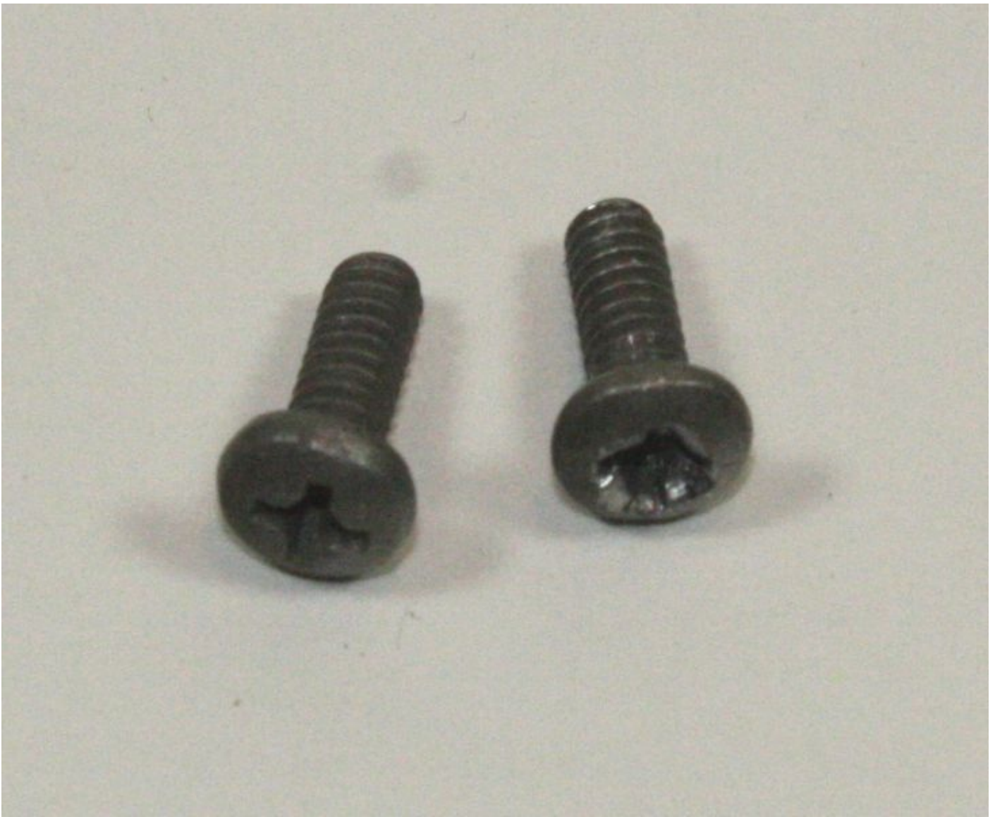
Figure 4-4. Damaged Phillips screw
