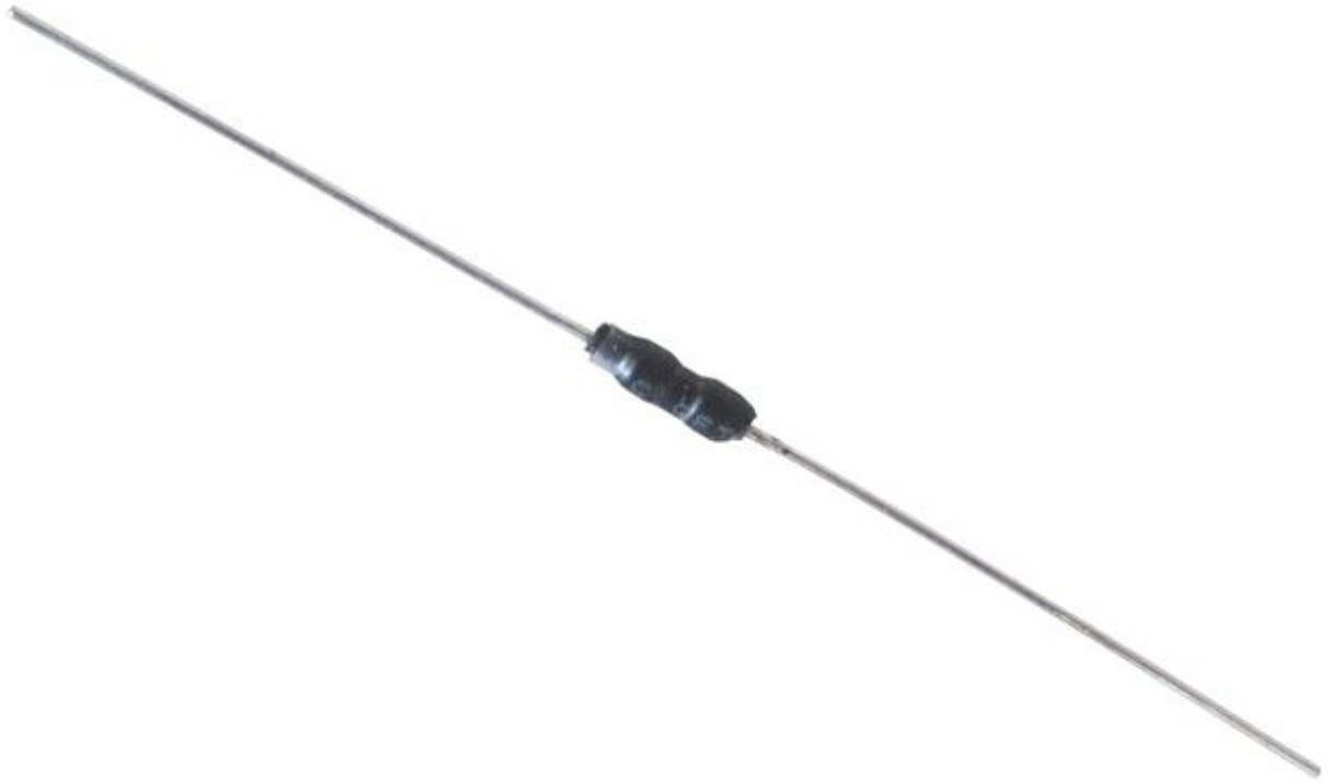
Figure 5-25. Printed circuit board-mounted fuses
