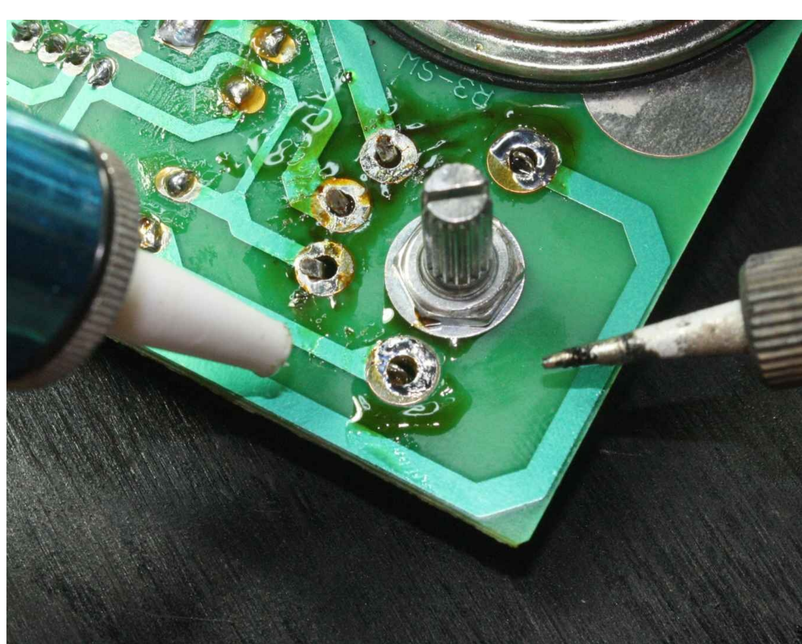
Figure 4-38. Result of using a solder pump on a large pad
