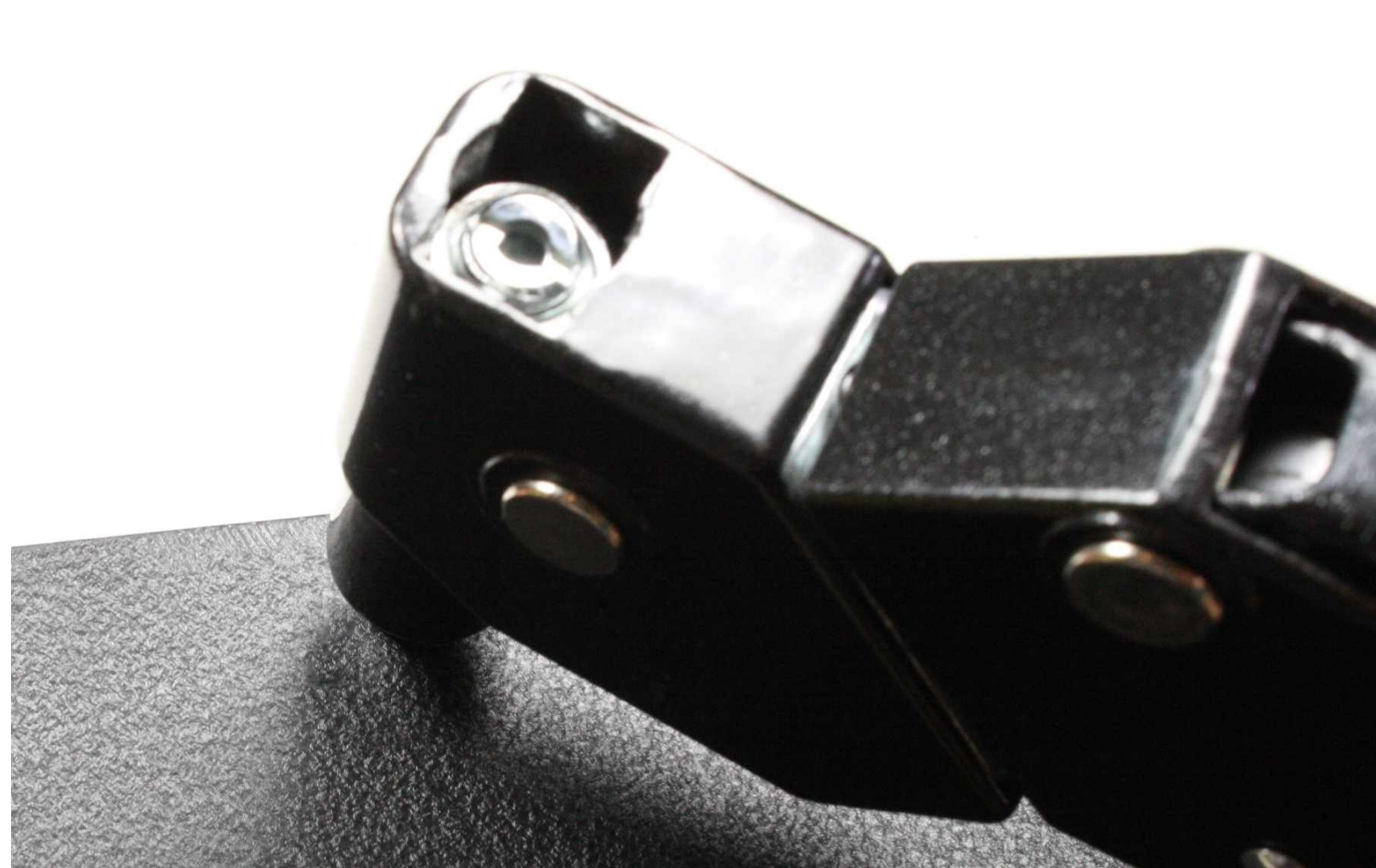
Figure 4-20. Installing a blind rivet: setting the rivet
