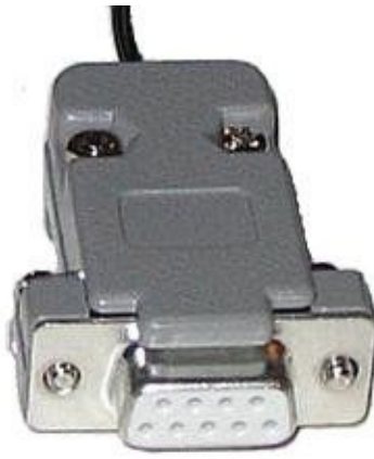
Figure 7-28. DB-9 connector with backshell
