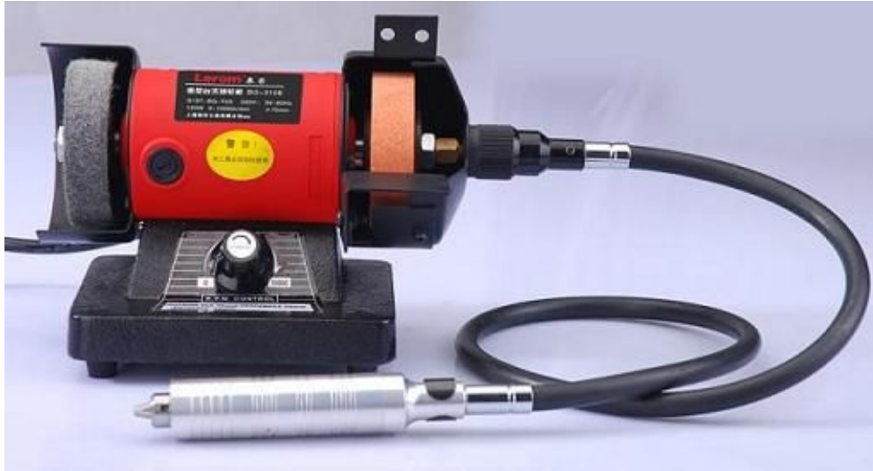
Figure 3-26. Small bench grinder with rotary tool attachment
