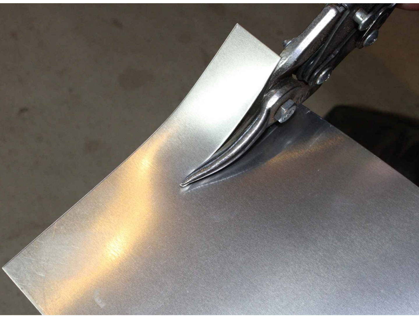
Figure 4-54. Using aircraft-style metal shears
