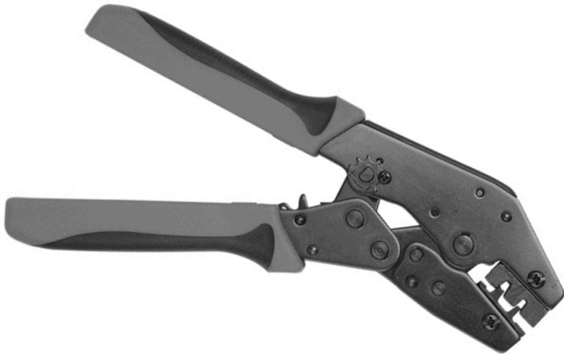
Figure 3-11. A crimping tool for small contacts
