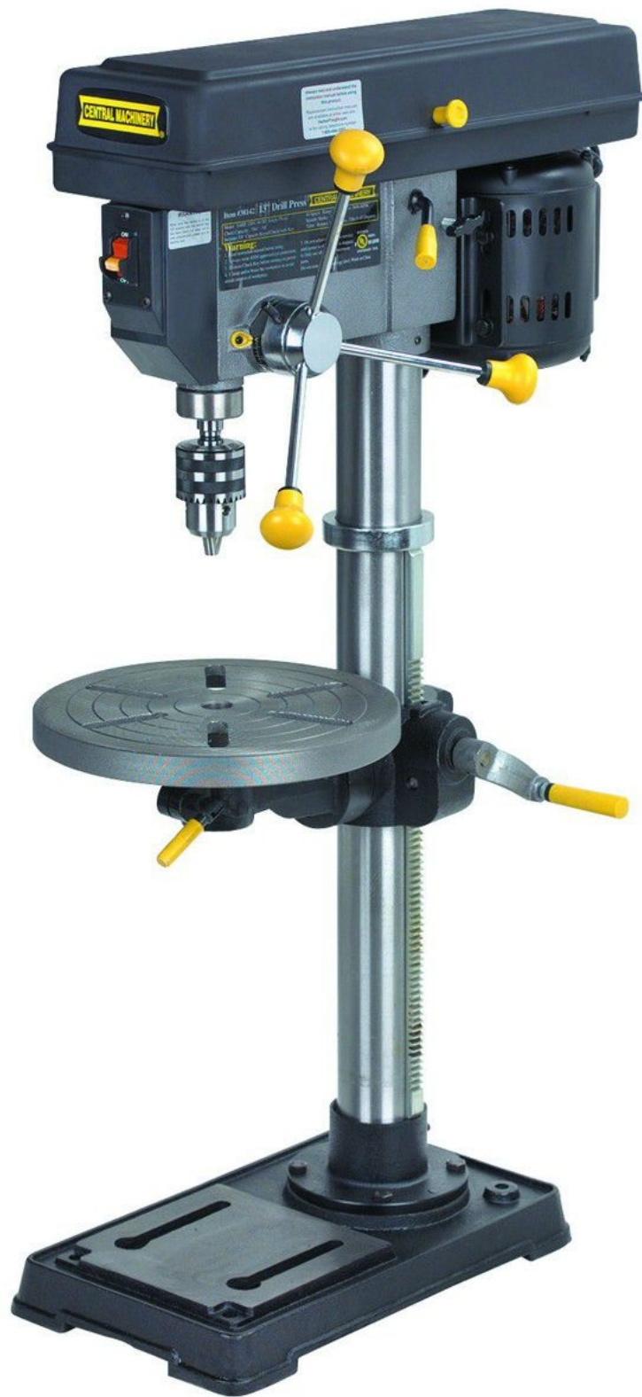
Figure 3-29. Small bench-top drill press
