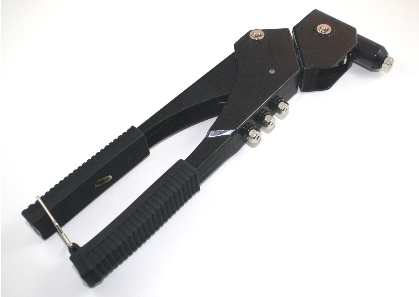
Figure 2-10. Hand-operated blind rivet installation tool
