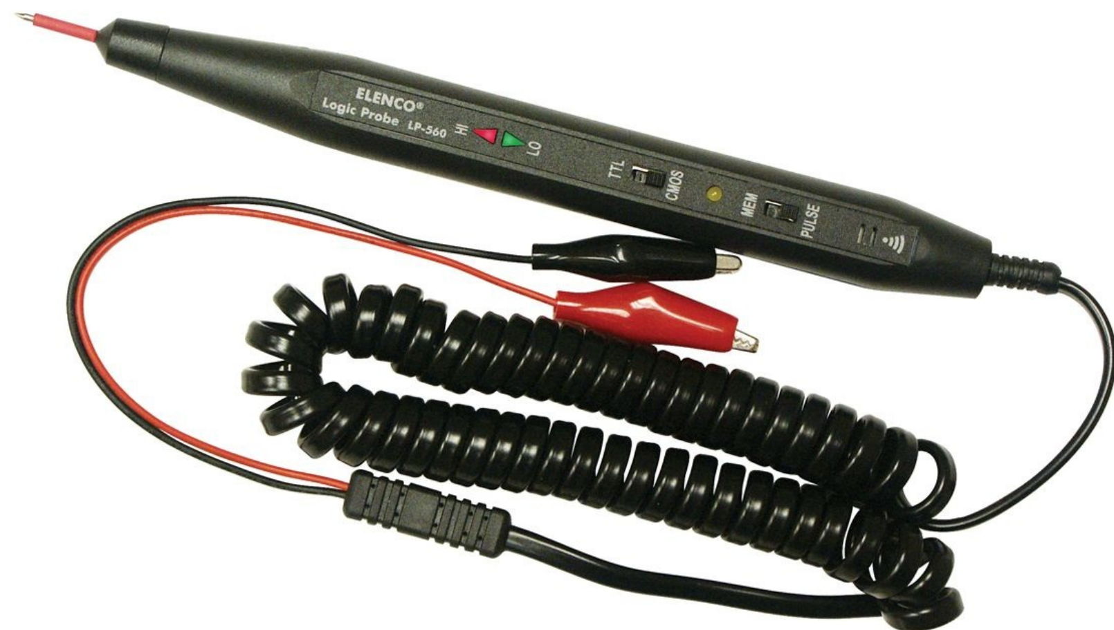
Figure 11-7. Hand-held digital logic probe
