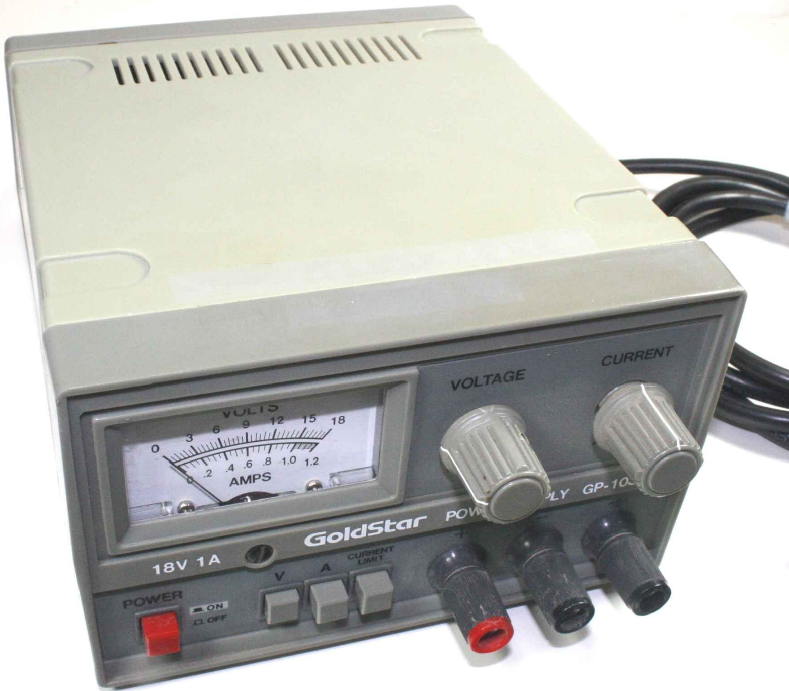
Figure 5-18. Variable-output bench DC power supply
