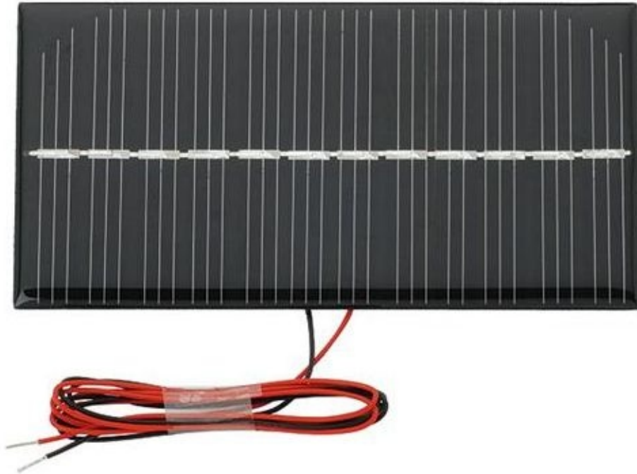
Figure 5-22. A small solar-cell module
