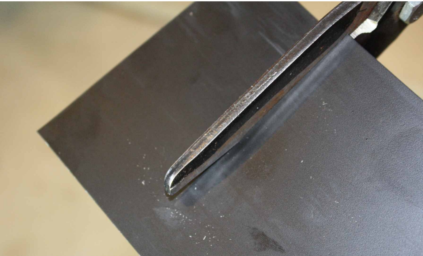
Figure 4-52. Using shop shears on sheet plastic
