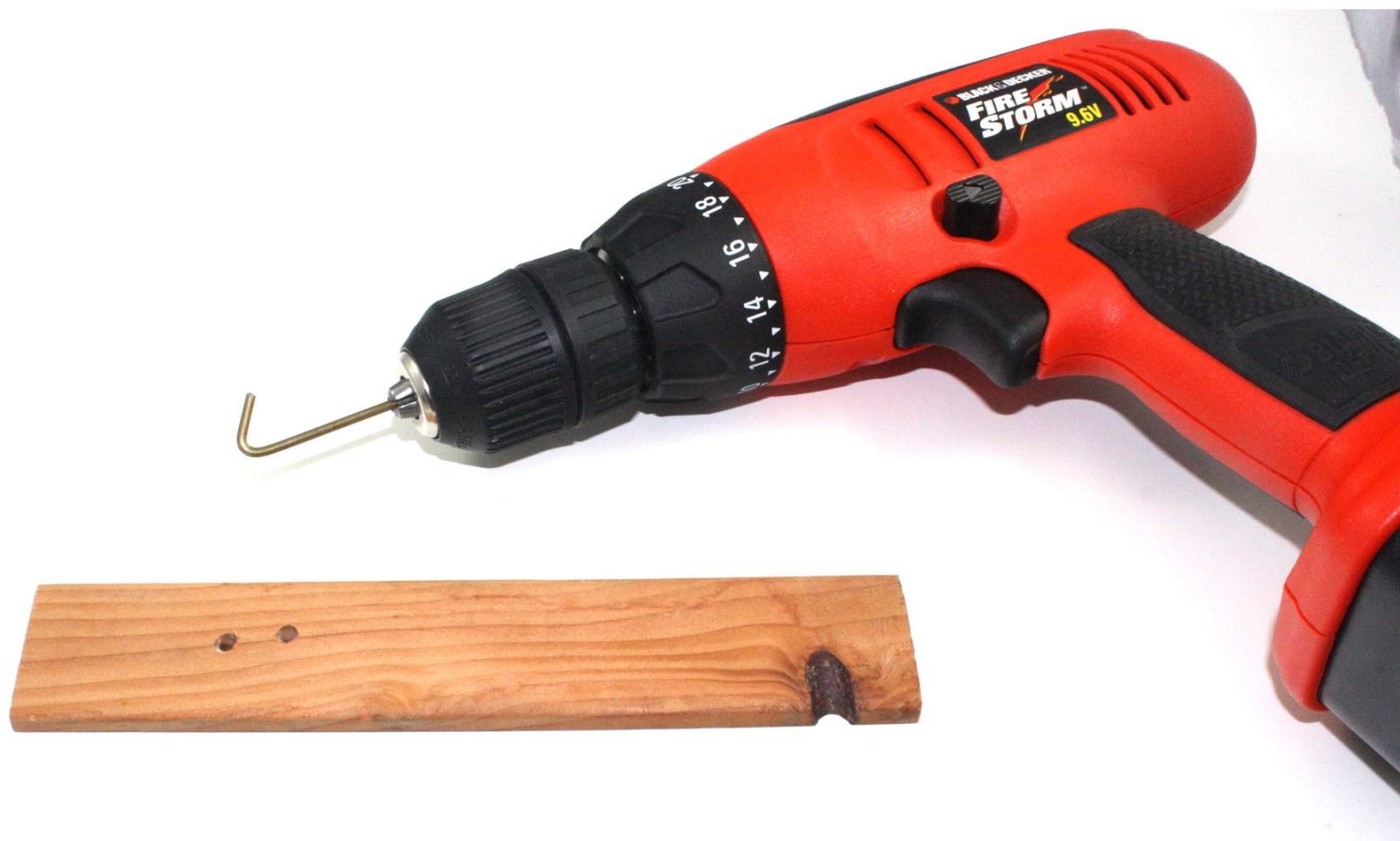
Figure 7-6. Improvised hook and guide board for making twisted-pair wire
