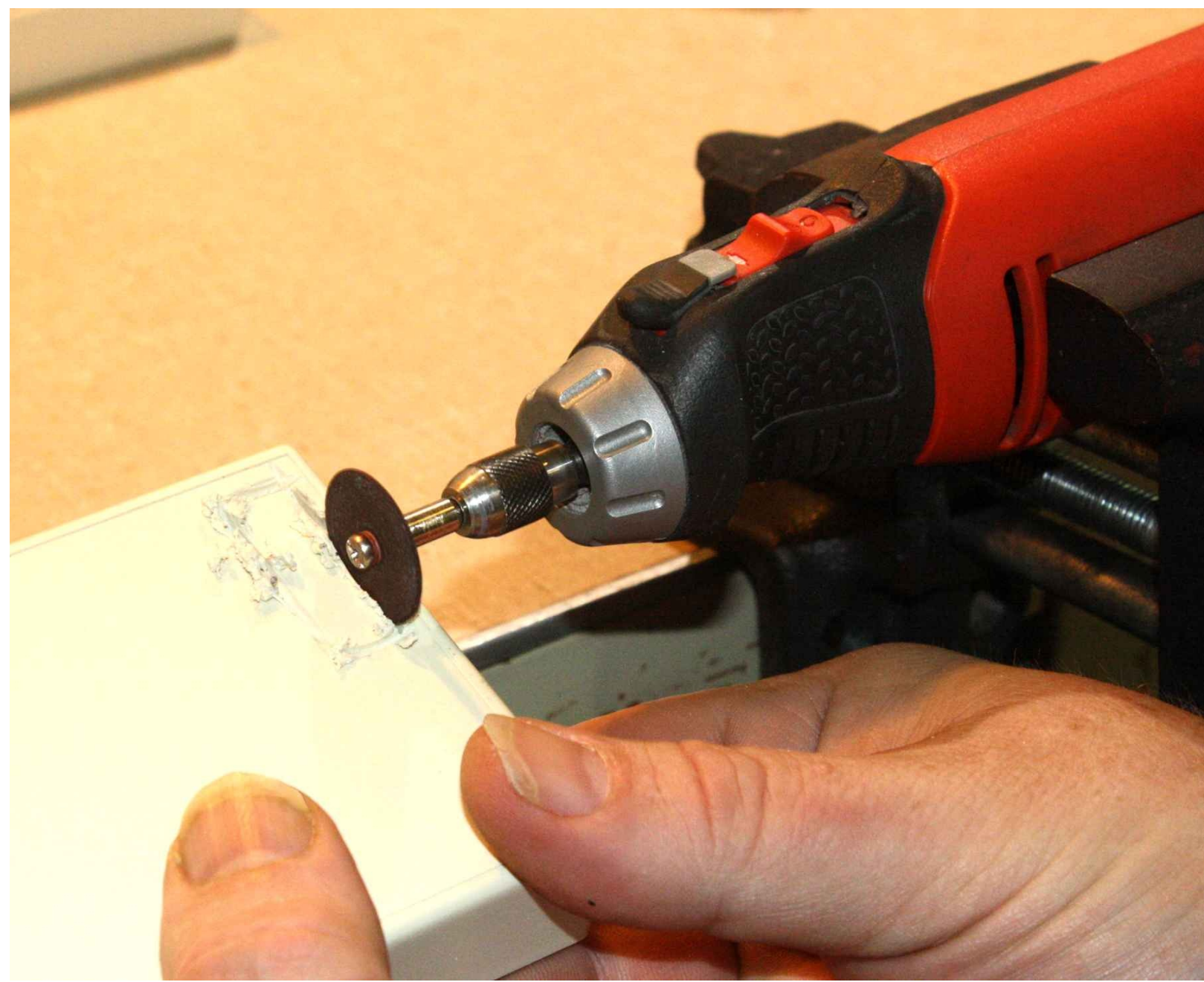
Figure 4-71. Rotary tool in a bench vise
