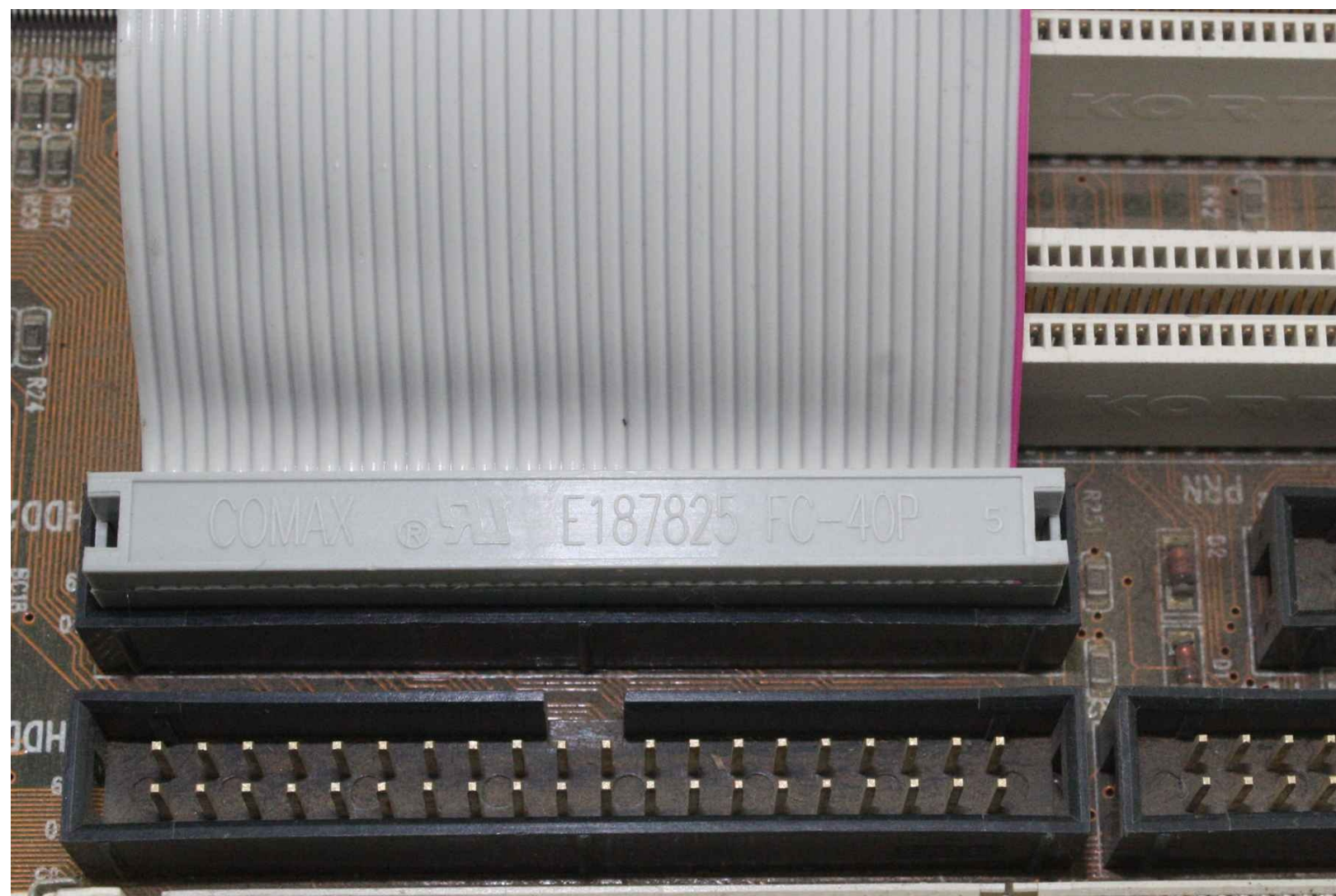
Figure 7-20. Ribbon cable with an IDC and a PCB-mounted header
