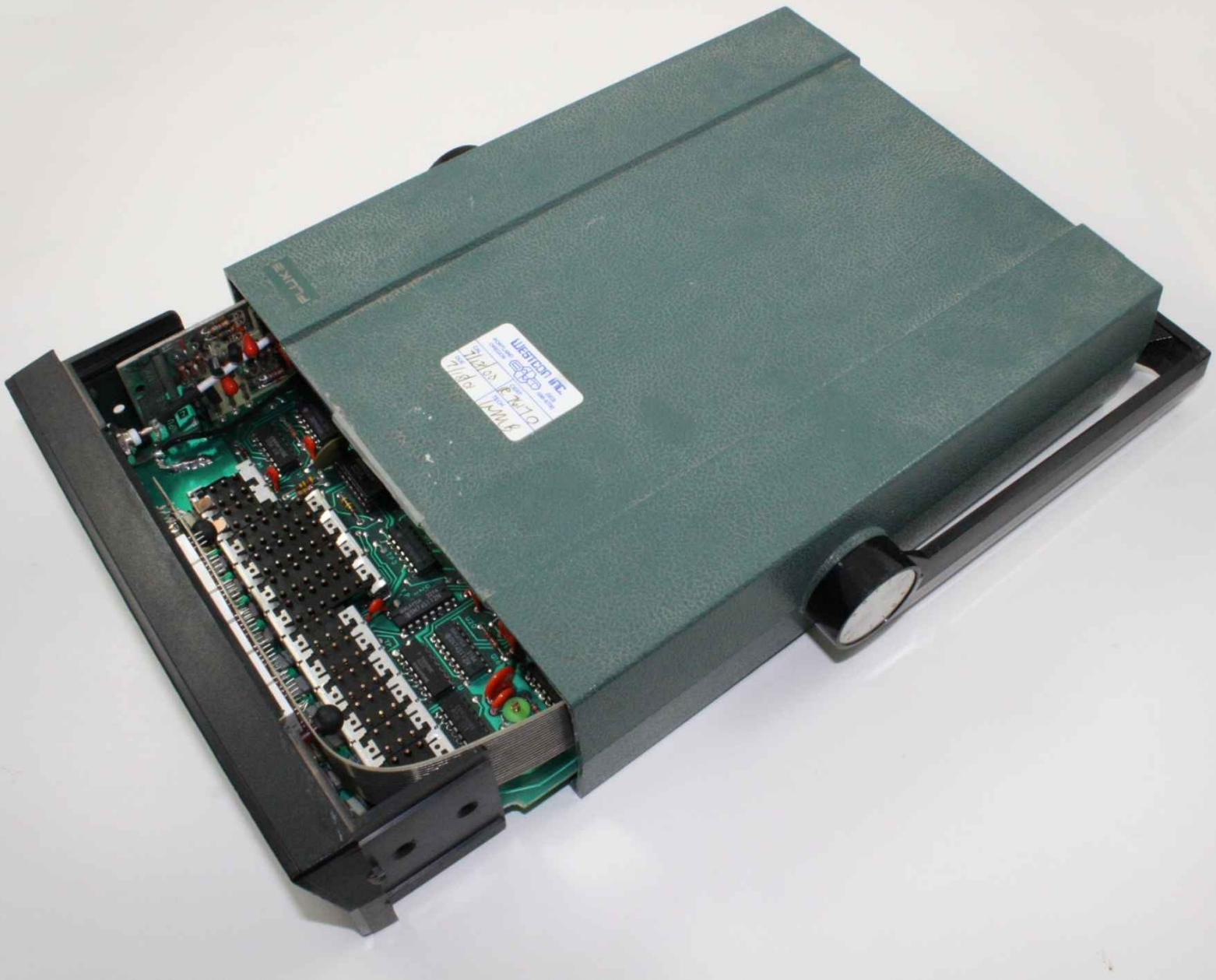
Figure 16-18. Fluke two-part plastic instrument enclosure with carry handle
