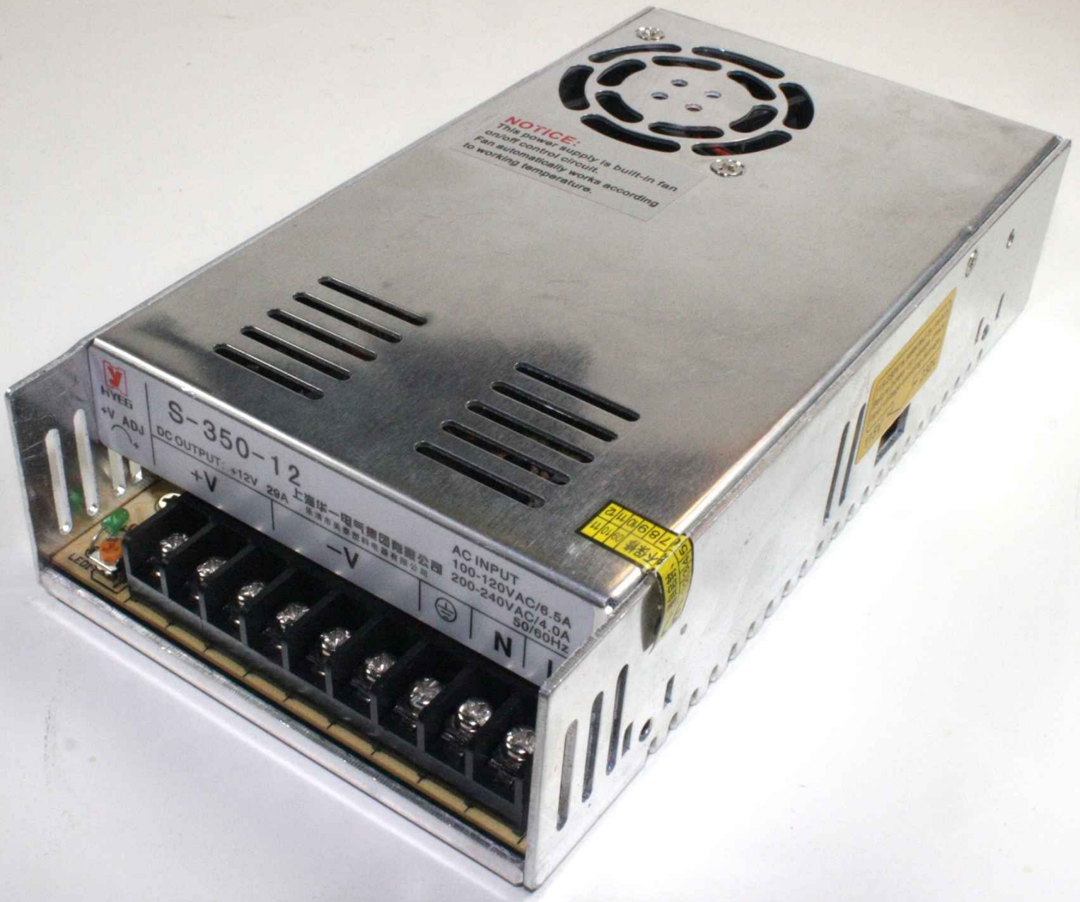
Figure 5-19. Modular 12V DC switching power supply
