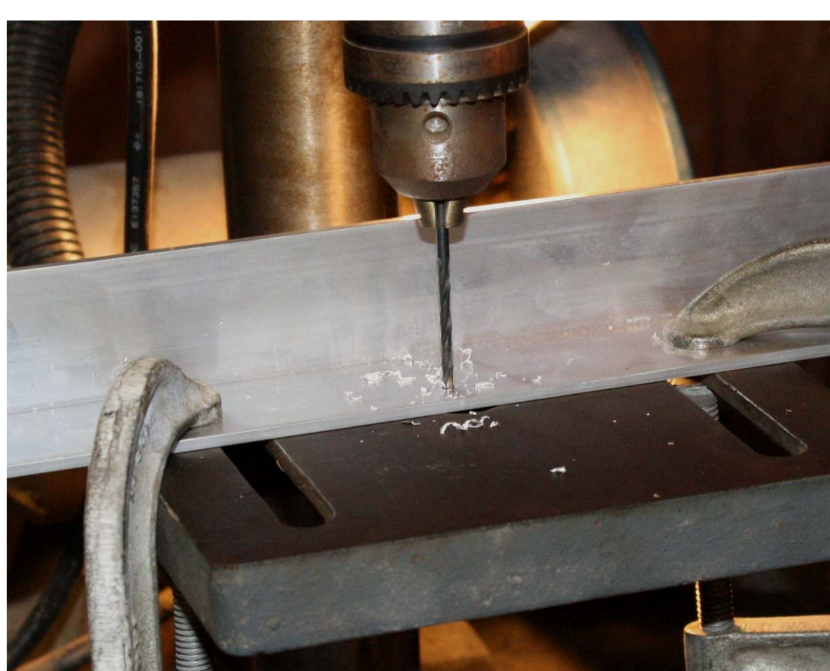
Figure 4-59. Drilling a hole for tapping with a drill press
