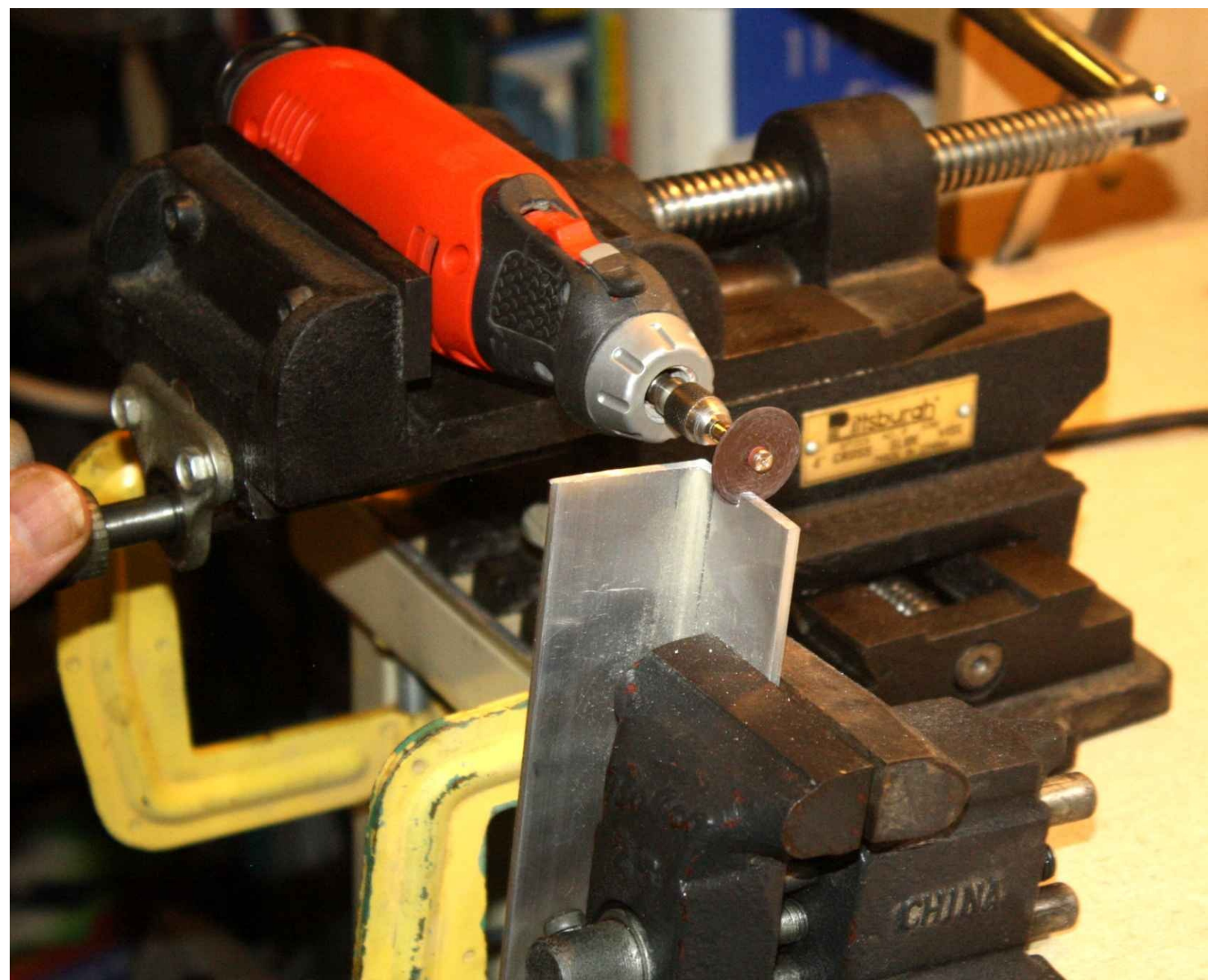
Figure 4-72. Holding a rotary tool in an X-Y cross-slide vise
