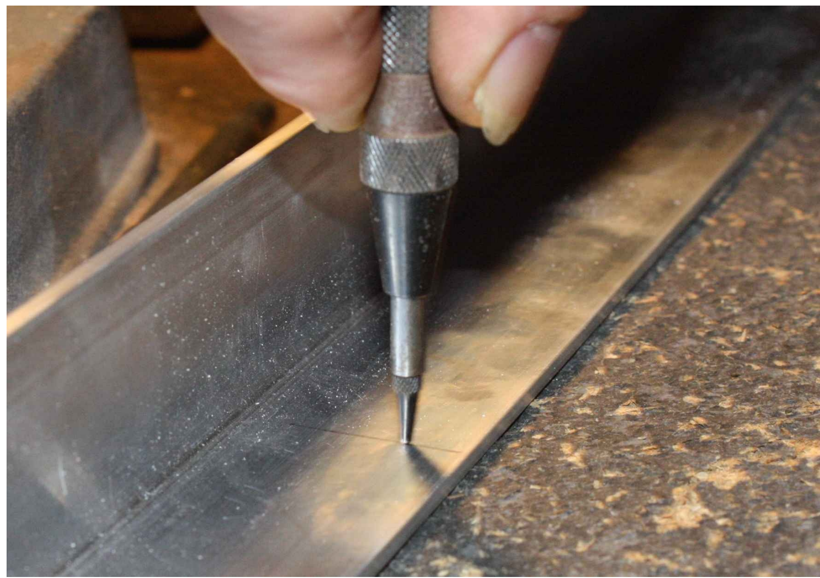
Figure 4-58. Preparing to drill a hole for tapping
