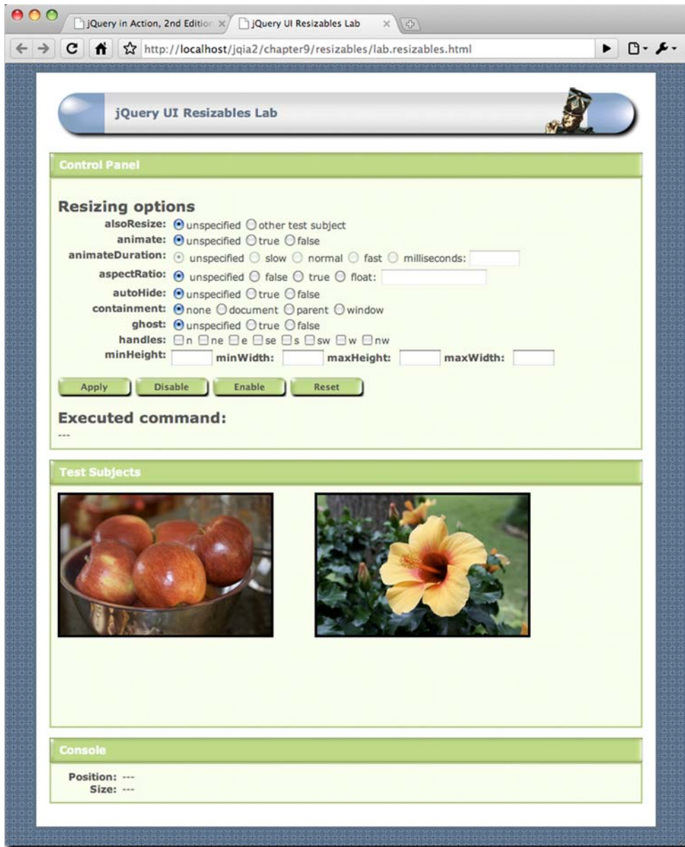
Figure 10.5 The Resizables Lab lets us see the operation of the various resizability options in action.
