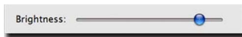
Figure 11.5 Sliders can be used to represent a range of values; in this example, from minimum to full brightness.
