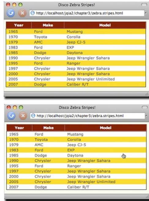
Figure 3.2 The presence or absence of the striped class is toggled whenever the mouse cursor enters or leaves the table.
