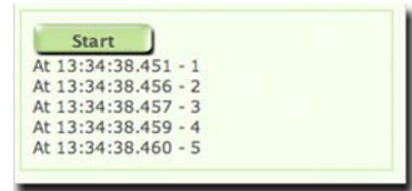
Figure 5.7 The console messages appear in rapid succession, proving that the animation methods aren’t blocking until completion.
