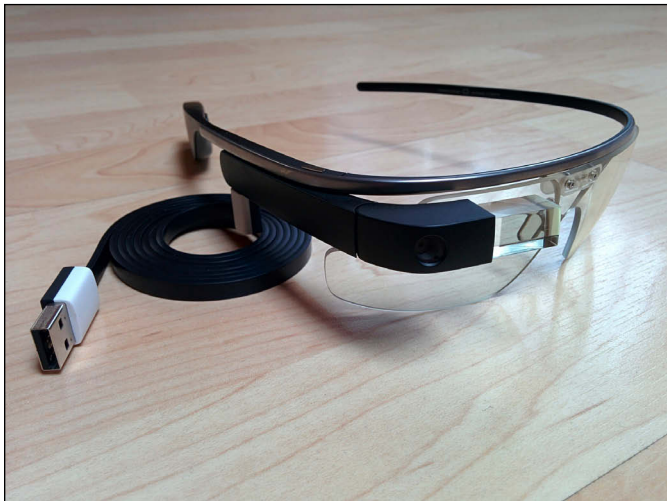
Figure 16-3: One side of the cable port is white, to plug into the charger; the other side plugs into the Glass device.
