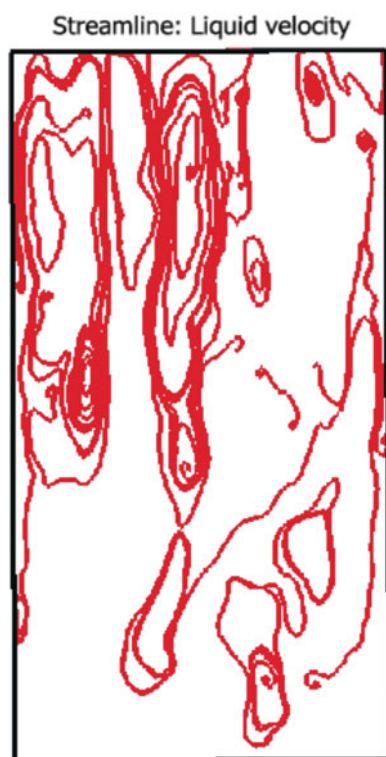
Fig. 13.3 CFD simulation of a plate photobioreactor of 1 m height; even moderate aeration leads to sufficient axial mixing ( T_{\text{mix}} \approx 100 s) as indicated by the streamlines
