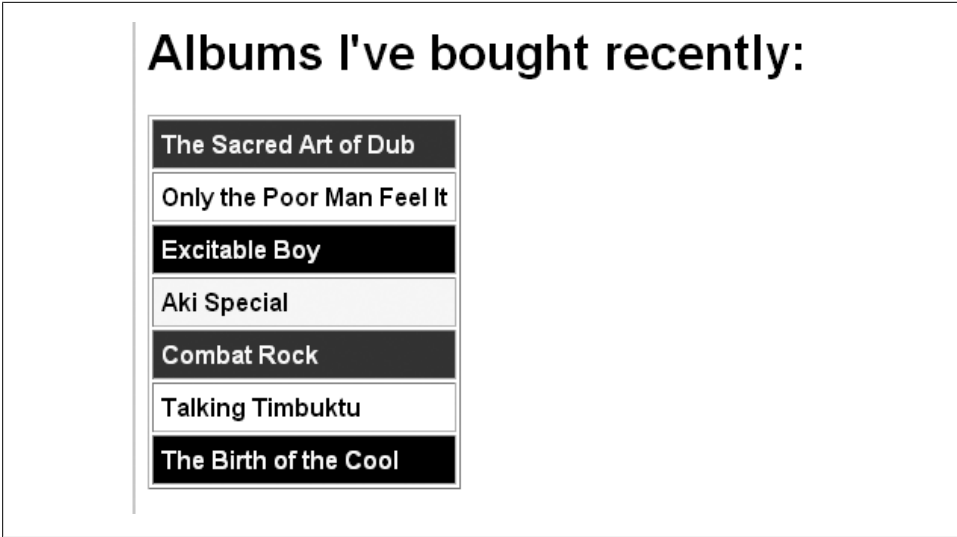
Figure A-17. Generating different background colors with <xsl:when>
