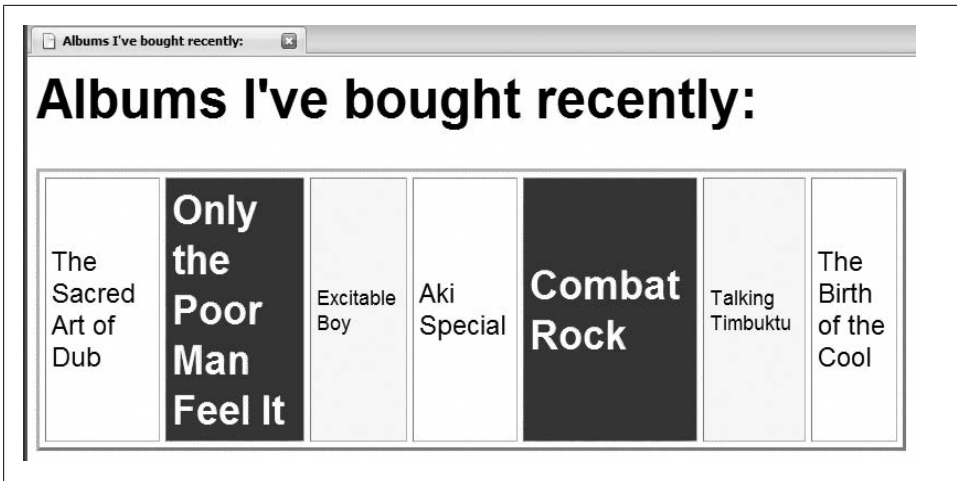
Figure A-10. An HTML table generated with the help of XSLT functions
