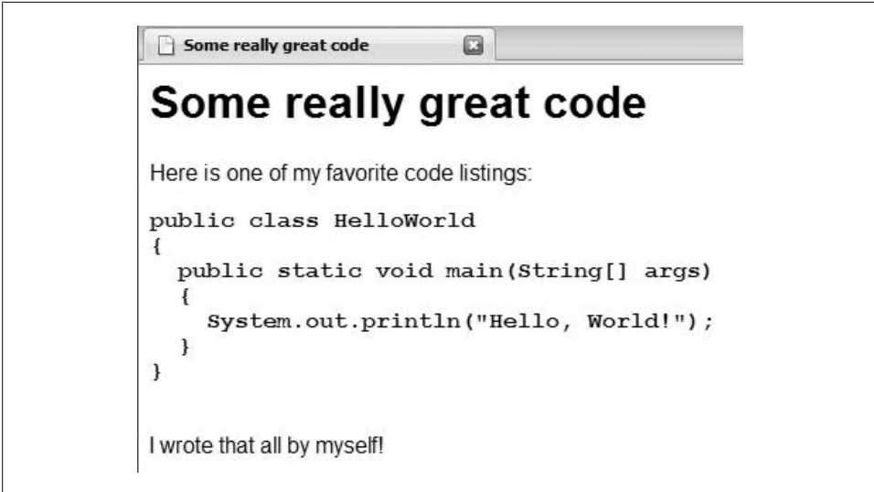
Figure A-1. HTML generated using a template imported from another stylesheet
