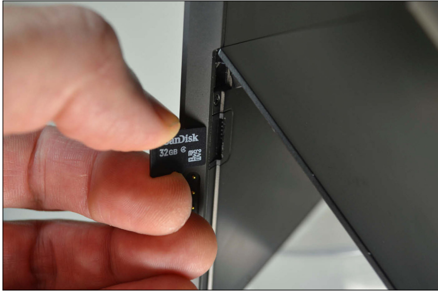
Figure 6-18: Push the card into the slot until it locks into place.
