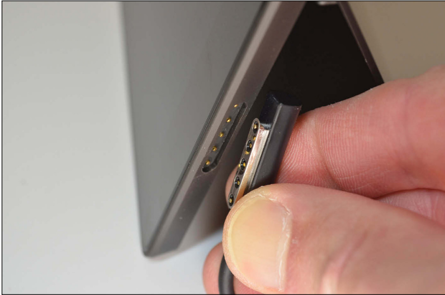
Figure 2-3: The symmetrical connector fits into the charger socket either way.
