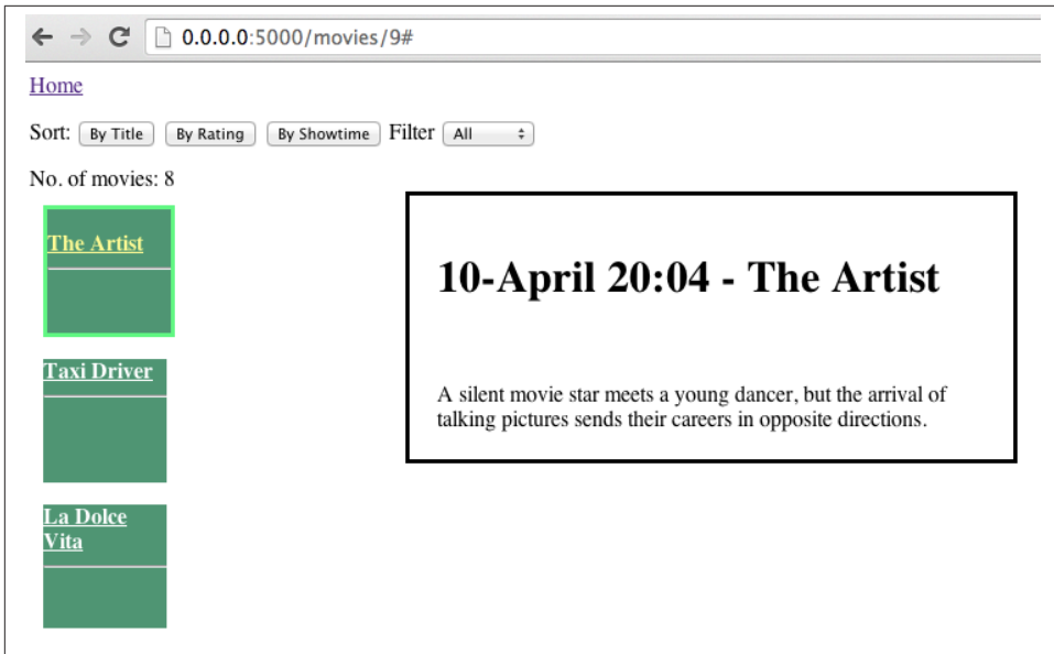
Figure 5-2. We can now filter and sort movies in the UI; for sorting, we keep all models in a collection, but models are removed for filtering, and we need to save a copy of the original collection
