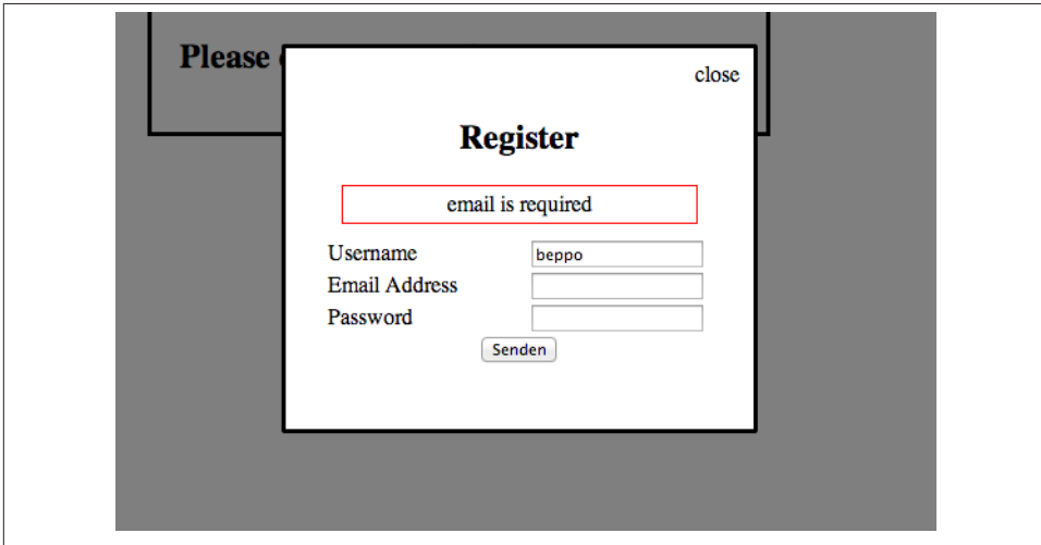
Figure 9-2. The view for signup is a custom modal view and handles errors from the validation of the UserModel
