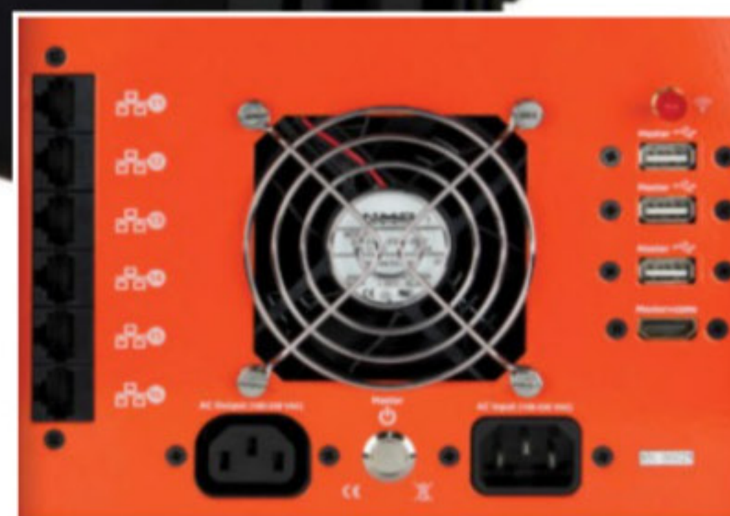
■ The Ubuntu Orange Box packs in ten NUC-based cluster nodes, has 40 logical processing cores and 160GB of RAM
