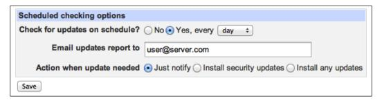
**cron** is a system utility, which runs in the background as a daemon and starts tasks that are scheduled to execute at a specific time. When **Scheduled checking options** is enabled, Webmin adds an entry in the system's cron table to execute its update verification script. The cron daemon will then execute the script once every day (hour or week, depending on the setting). If Webmin discovers available updates, it will send you an e-mail.
