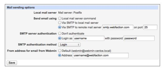
5. Go back to **Webmin | Webmin Configuration | Sending Email**, and use the **Send test message** form to test your configuration.
