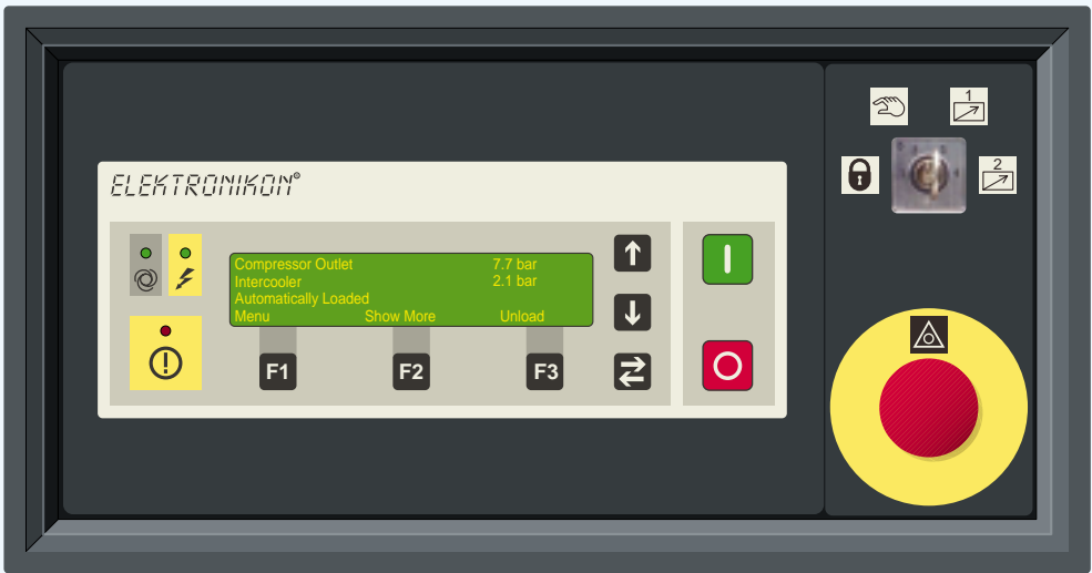
A user-friendly monitoring panel shows all the operating parameters for the compressor, for example, pressure and temperatures, with data logically grouped for direct read-off.
