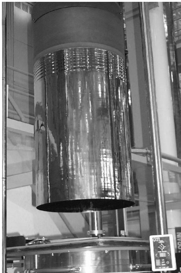
Figure 6.23 Experimental 50-cm-diameter EFG cylinder exiting from furnace
