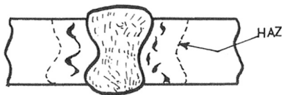
FIGURE 6.24 Crack patterns under stress relief.
