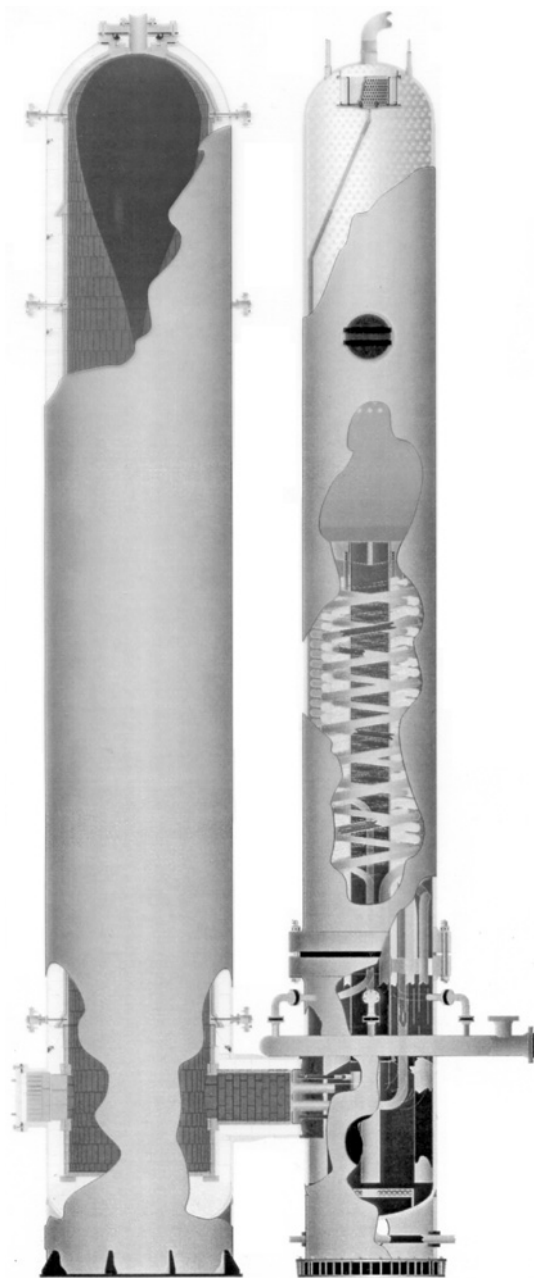
Figure 5.33 Shell reactor and syngas cooler (source: de Graaf et al. , 2000; reproduced with permission from Shell).
