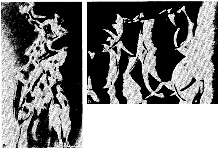
Fig. 35. Short durations in Schlieren photographs of open turbulent flames [after Fox and Weinburg, Proc. R. Soc. London A 268 , 222 (1962)].
