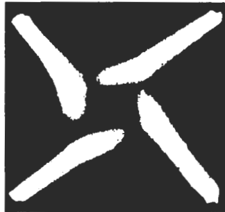
Plate 5.1: Direct flame photograph ( A/F = 17 , \theta = 6^\circ ) [932].
