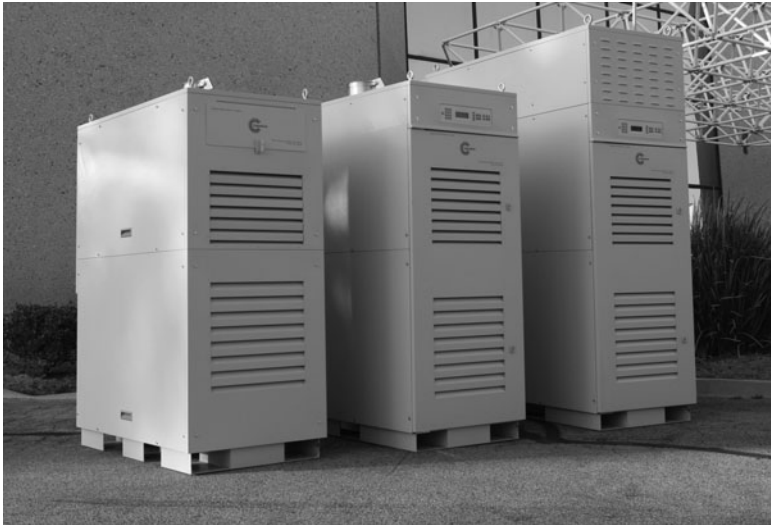
FIGURE 6-14 Capstone microturbine 30 kW (left), 65 kW (center), and 65 kW with integrated CHP for hot water supply (right) units in upper photo; lower image is cutaway of 65 kW turbine components. Module on top of right unit recovers heat from turbine to generate hot water for space heating or DHW. (Images: Capstone Turbine Corp. Reprinted with permission.)
