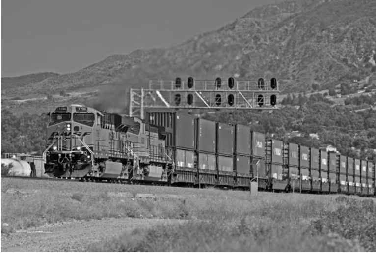
FIGURE 14-15 Double-stack intermodal train carrying shipping containers. (Photo: BNSF Railroad. Reprinted with permission.)
