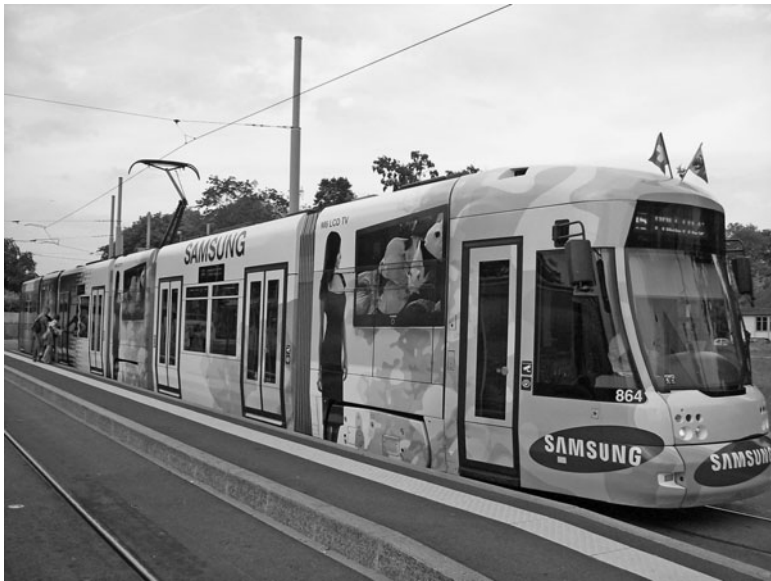
FIGURE 14-11 Bombardier “Flexity” Light-rail transit (LRT) vehicle at a stop in Geneva, Switzerland. In recent years the LRT railcar industry has pushed the maximum length of LRT vehicles while still allowing them to navigate street traffic where necessary. This development increases both maximum passenger capacity during peak periods and financial productivity of the asset, since the driver’s wages are distributed among a larger passenger base, all other things equal.
