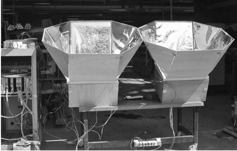
FIGURE 11-9 Solar ovens with four reflective sides undergoing parametric testing at Cornell University, May 2004.
