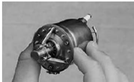
FIGURE 3 Microturbine designed for the Defense Advanced Research Projects Agency by M-Dot Aerospace. (Source: DARPA website.)
