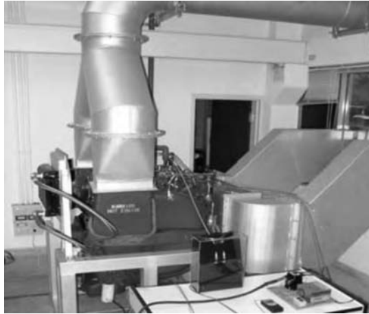
FIGURE 6-11 Microturbine engine test stand. (Source: Chiang, H.-W. D., Wang, C.-H., and Hsu, C.-N. 2004. Performance testing of a microturbine generator set with twin rotating disk regenerators . Proceedings of ASME Turbo Expo 2004. American Society of Mechanical Engineers. Vienna, Austria.)
