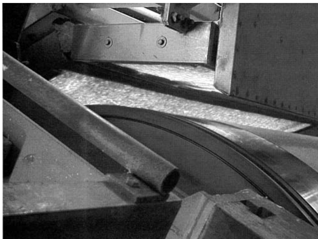
Figure 17.10 Supplemental IR burners for paper drying located over steam cylinders. (Courtesy of Marsden, Inc., Pennsauken, NJ.)
