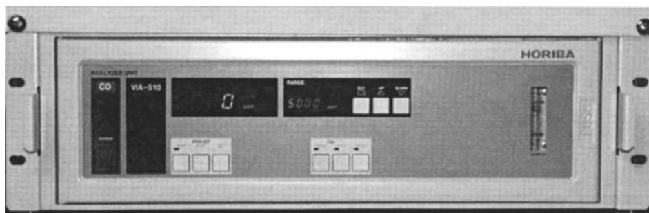
Figure 7.8 Nondispersive IR CO analyzer.
