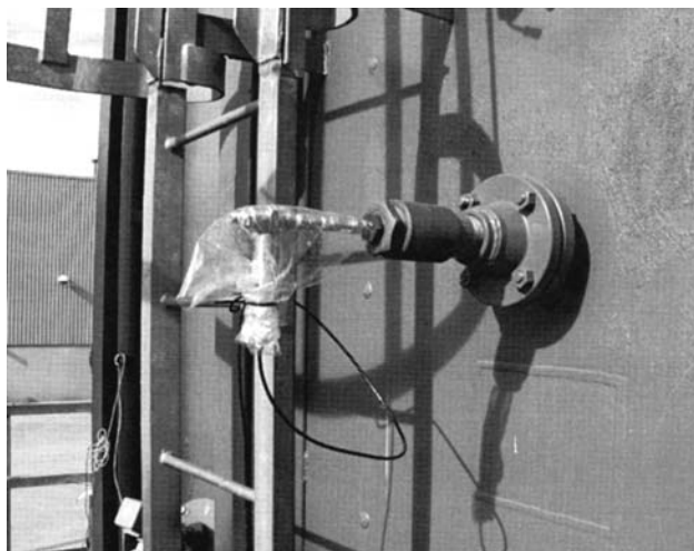
Figure 10.29 Vibration transducer on a furnace. (Courtesy of John Zink Co., Tulsa, OK.)
