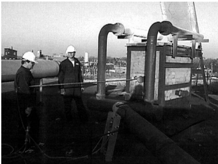
Figure 5.45 Measuring emissions from an exhaust stack.
