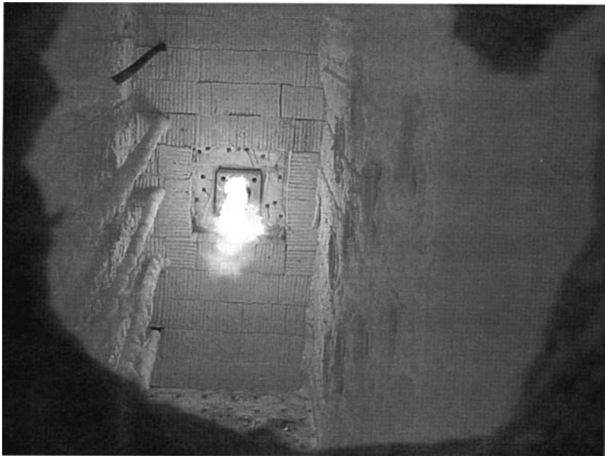
Figure 12.14 Downfired burner with liquid naphtha fuel. (Courtesy of John Zink Co. LLC, Tulsa, OK.)
