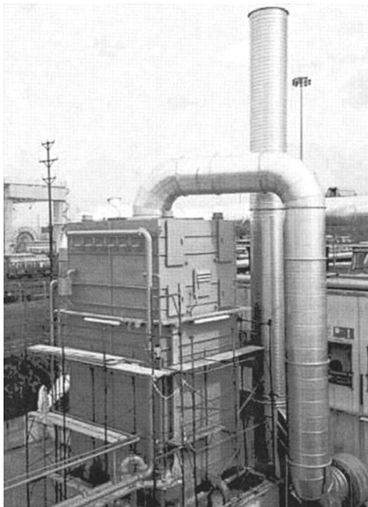
Figure 9.21 Industrial wet electrostatic precipitator. (Courtesy of Croll.)
