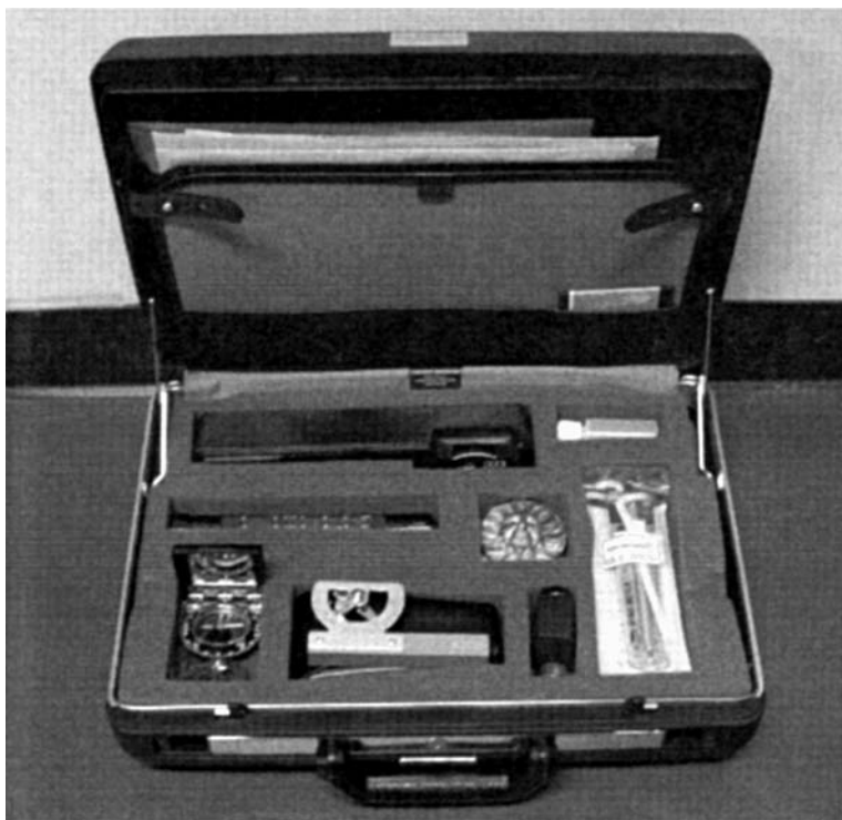
Figure 5.49 Field kit for making gas emission measurements. (Courtesy of ETA, Garner, NC.)
