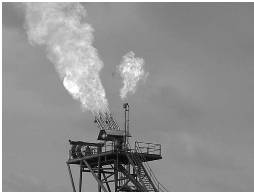
Figure 1.16 Flare on an offshore oil platform with water injection for thermal radiation suppression. (Courtesy of John Zink Co., Tulsa, OK.)
