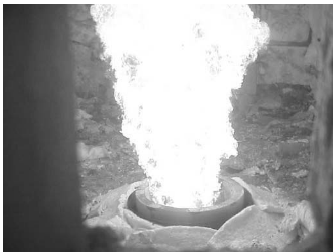
Figure 3.6 Example of a highly luminous heavy oil flame. (From Ref. 4. Courtesy of John Zink Co.)
