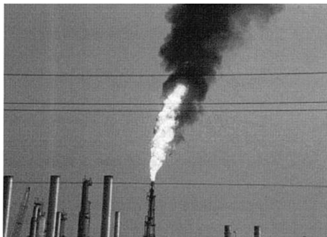
Figure 15.30 Typical elevated single-point flare. (From Ref. 63. Courtesy of John Zink Co. LLC.)
