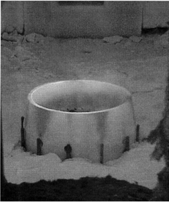
Figure 12.32 John Zink LM-300 burner incorporating furnace gas recirculation operating in a furnace. (Courtesy of John Zink Co. LLC, Tulsa, OK.)
