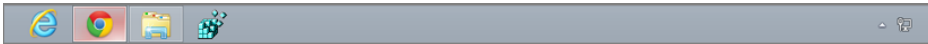
Figure 6-10: The Windows 8 taskbar shows applications that are running surrounded by a border.
