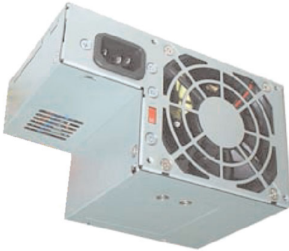
Figure 18.10 CFX12V power supply.
