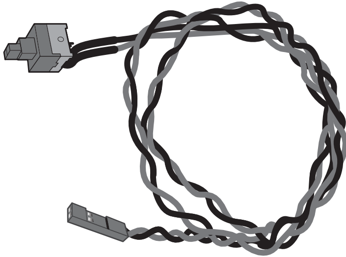
Figure 18.16 ATX power switch.
