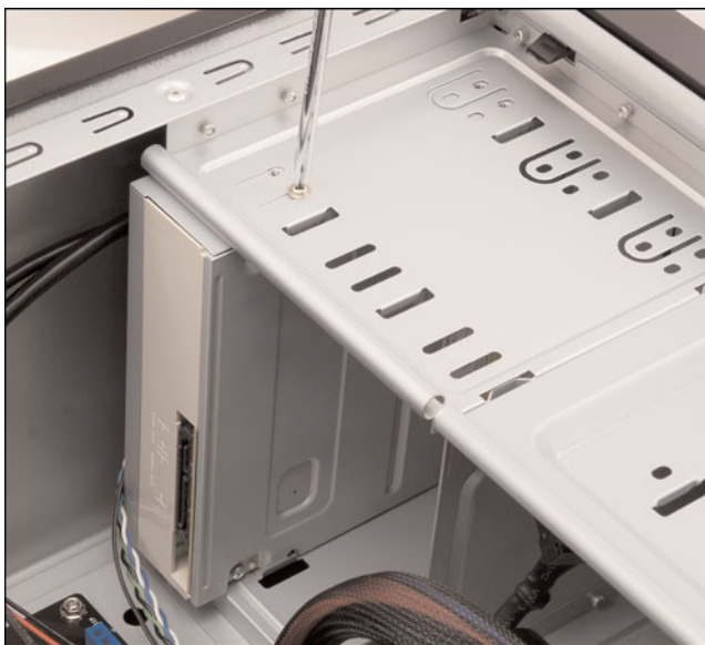
Figure 19.29 Secure the drive to the chassis using four screws, two on each side of the drive.
