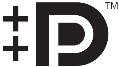
Figure 12.14 Icon indicating a DisplayPort with Multimode (DVI and HDMI) support (right).
