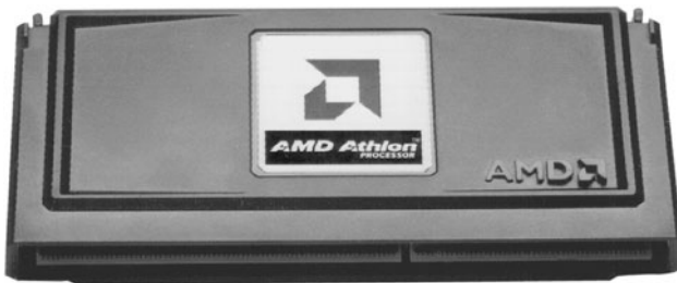
Figure 3.33 AMD Athlon processor for Slot A (cartridge form factor).
