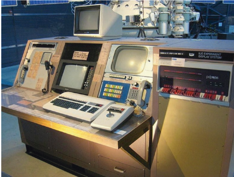
Figure 1-1. PDP 11/35, a microprogrammed successor to the PDP-11/20; the design team was led by Jim O’Loughlin
