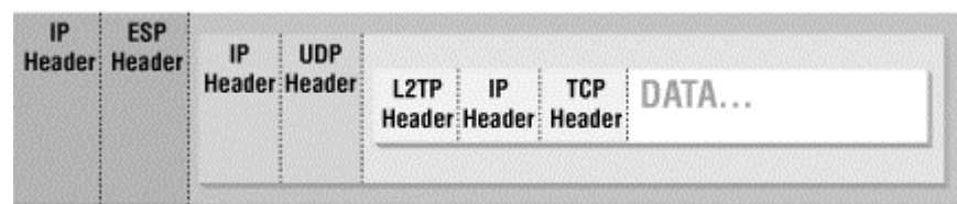
Figure 14.4. L2TP encapsulation of a TCP packet, as normally seen crossing an IP network
