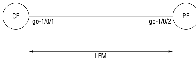
Figure 17-1: Configuring Ethernet LFM with remote loopback on a span.
