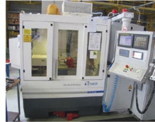
Studer S120 Year: 2007 Internal Grinding Wheel Spindle Motor Power: 10 kW Max RPM: 60000
