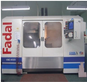
Fadal VMC4020 Year: 1998 Axes No.: 3 Spindle No.: 1 Motor Power: 11 kW
