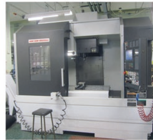
Mori Seiki Dura Vertical 5100 Year: 2008 Axes No.: 3 Spindle No.: 1 Motor Power: 15 kW
