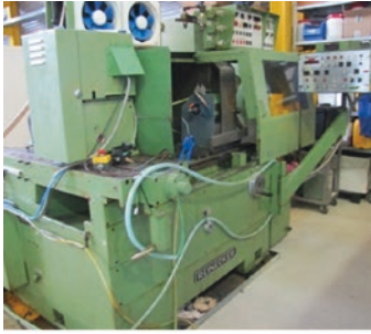
Studer S120 Year: 2007 Internal Grinding Wheel Spindle Motor Power: 10 kW Max RPM: 60000
