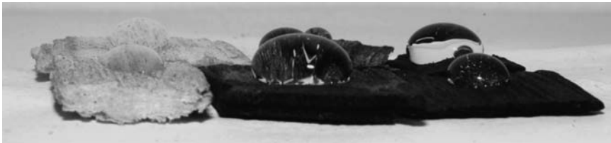
Figure 7.10. Illustration of the water resistance of torrefied (hydrophobic) material (right), compared to original (hydrophilic) wood chips (left) after one hour of exposure to water droplets.
