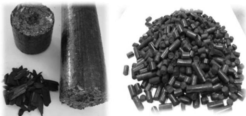
Figure 7.16. Torrefied and densified Norway spruce: briquettes (left) and pellets (right).
