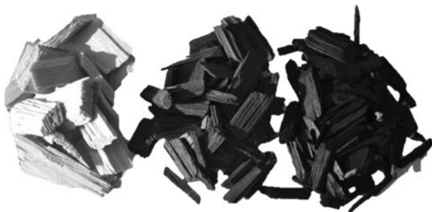
Figure 7.1. Original wood chips (left) and corresponding torrefied materials; light brown (center) and dark brown (right) subjected to 8 minutes at 260°C and 16.5 minutes at 285°C, respectively.
