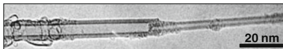
Fig. 2.18 TEM image of partially nested nanotubes after relative translation. Attractive forces pull back the nanotube to its nested initial position. (reprinted with permission [72])
