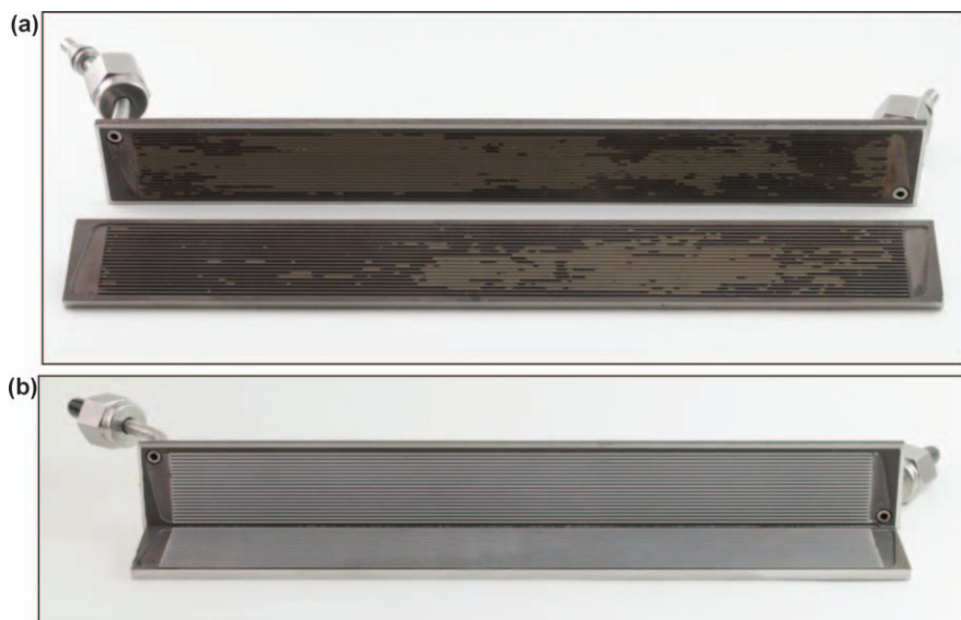
Figure 3.12 (a) Opened microreactor, which was tested for its activity in galactose to galactitol hydrogenation. Operational conditions: T = 105^{\circ}\text{C} , p = 60 bar, gas to liquid ratios varying from 1 to 20\text{ (mL min}^{-1}\text{)} . Sugar solution: galactose 0.23\text{ mol L}^{-1} . (b) Opened unused microreactor.
