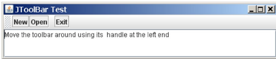
Figure 2-23. A JToolBar with three JButtons placed in the north region of a JFrame
