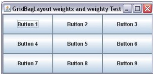
Figure 1-42. A JFrame with a GridBagLayout having nine buttons after resizing. All buttons have their weightx and weighty set to 1. Extra space is distributed among the display area of all buttons equally
