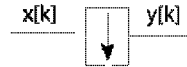
FIGURE 3.10: The discrete signal x[k] is downsampled by a factor of 2 by removing every other sample.
