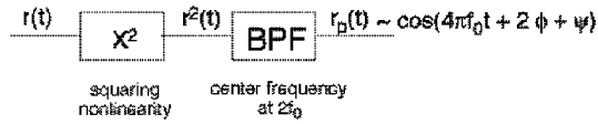
FIGURE 10.3: Preprocessing the input to a PLL via a squaring nonlinearity and BPF results in a sinusoidal signal at twice the frequency and with a phase offset of twice the original.
