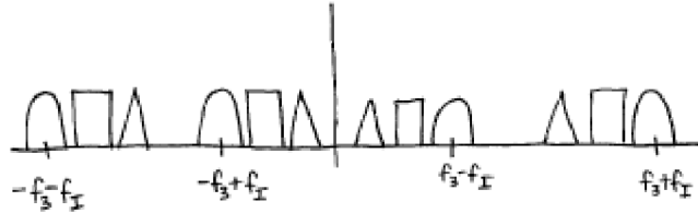
FIGURE 2.9: FDM Downconversion to an Intermediate Frequency
