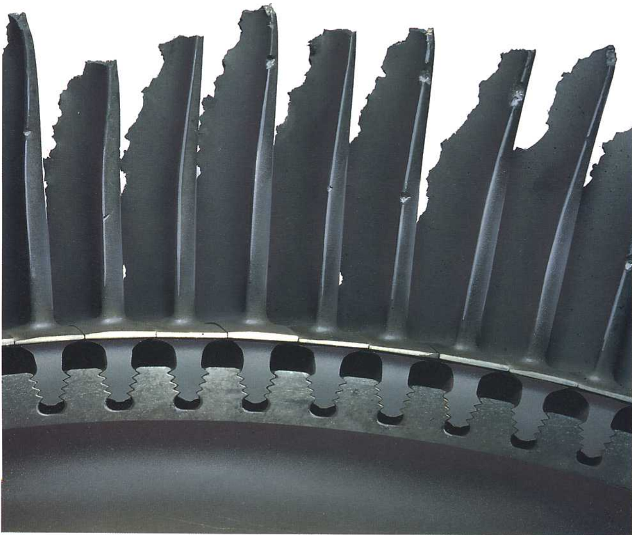
Fig. 24-9 Overheated turbine blades.
