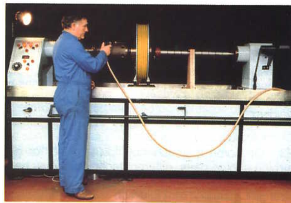
Fig. 25-3 Magnetic crack testing.
