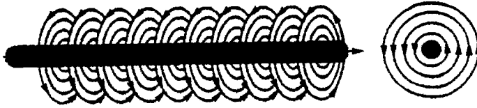
Figure 15.30—Magnetic Field Around a Conductor Carrying Current
