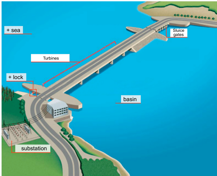
FIGURE 9.1 A tidal barrage power plant.
